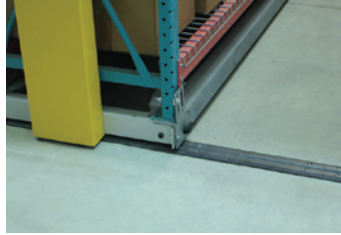
Shown are the surface-mounted rails used on Proteus Packaging's ActivRAC system.
