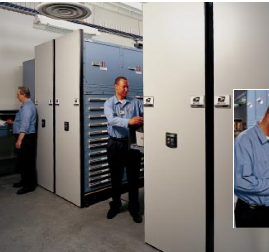
A programmable electric mobile system consolidated the parts storeroom and made space for new automated equipment.
